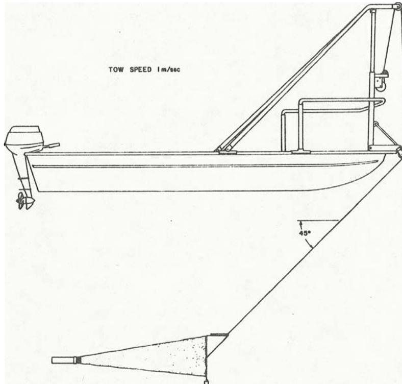
Figure 8. "Push" boat used by TVA in 1977 for larval fish sampling in shallow water (0.5 m) areas.
