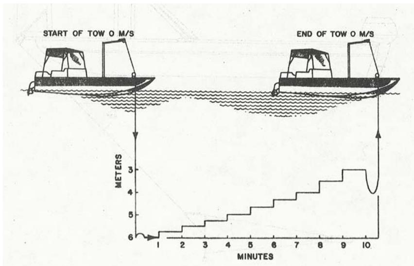
Figure 7. Open-water sampling boat and the "stairstep" retrieval pattern for stratified sampling.
