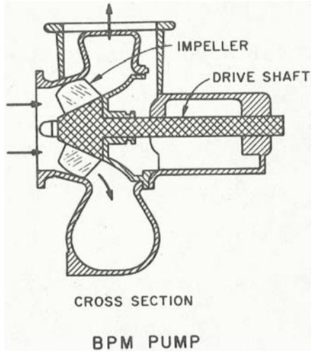
Figure 9. Cross section of a BPM pump.
