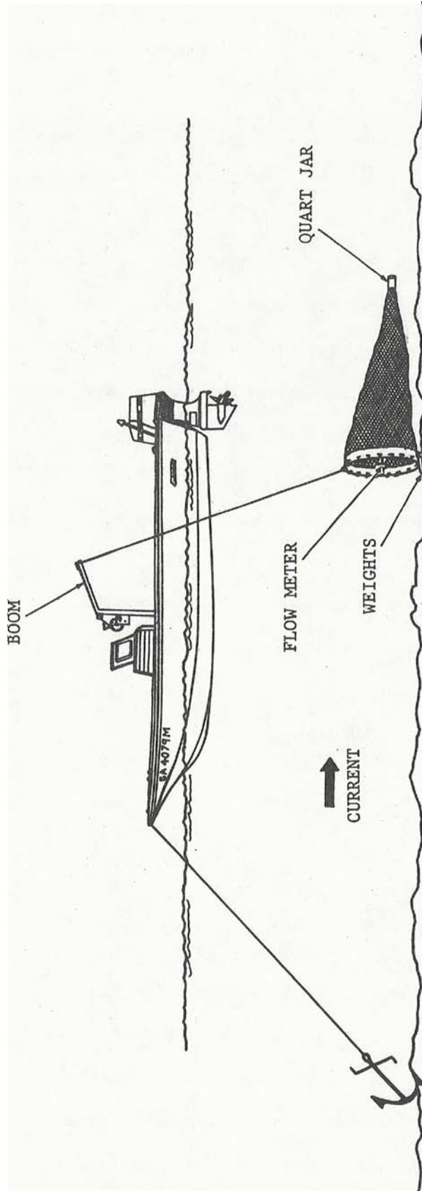
Figure 2. Diagram of ichthyoplankton sampling gear.
