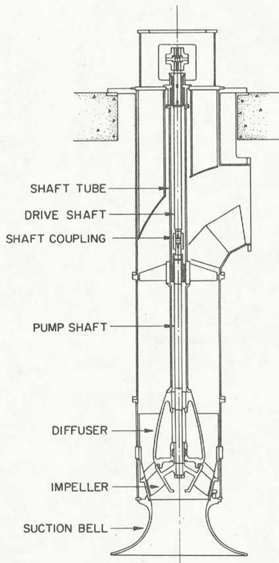
Typical Section View of Power Plant Circulating Water Pump.
