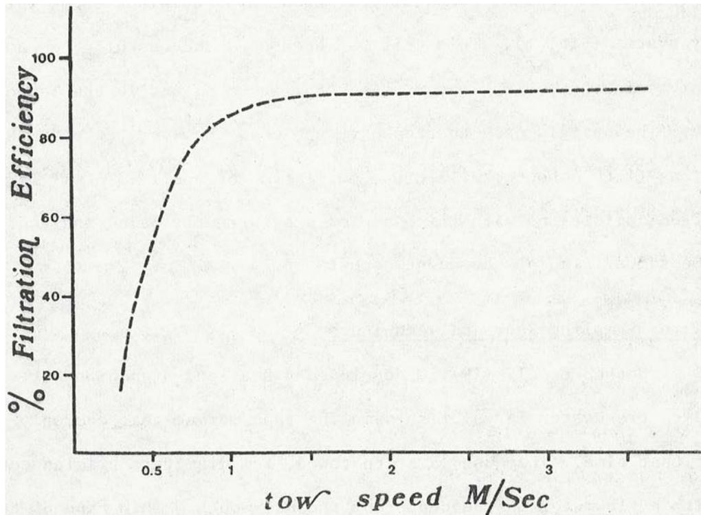
Figure 4. Filtration efficiency of a typical conical larval fish net\* (Svein Vigander, Tennessee Valley Authority, Water System Development Branch, 1976).
