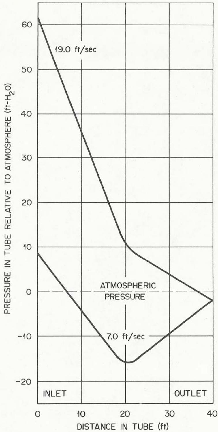
Figure 2. Pressure in tube relative to atmosphere (m H<sub>2</sub>O) (Kedl and Coutant, 1976).
