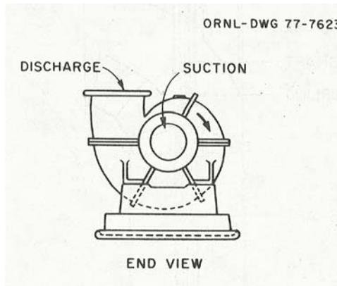
Figure 8. End view of a BPM pump.
