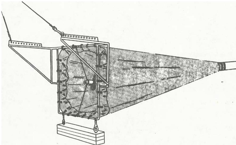
Figure 6. Net and frame of the side-towed larval fish sampler used by TVA in 1976-1977.
