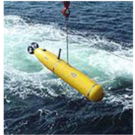
Picture of an autonomous underwater vehicle (AUV) taken by an employee of Bluefin Robotics Corporation during a US Navy exercise. An AUV will employed by the NCSU research team to help survey deep habitats for reef fish and crustaceans.
