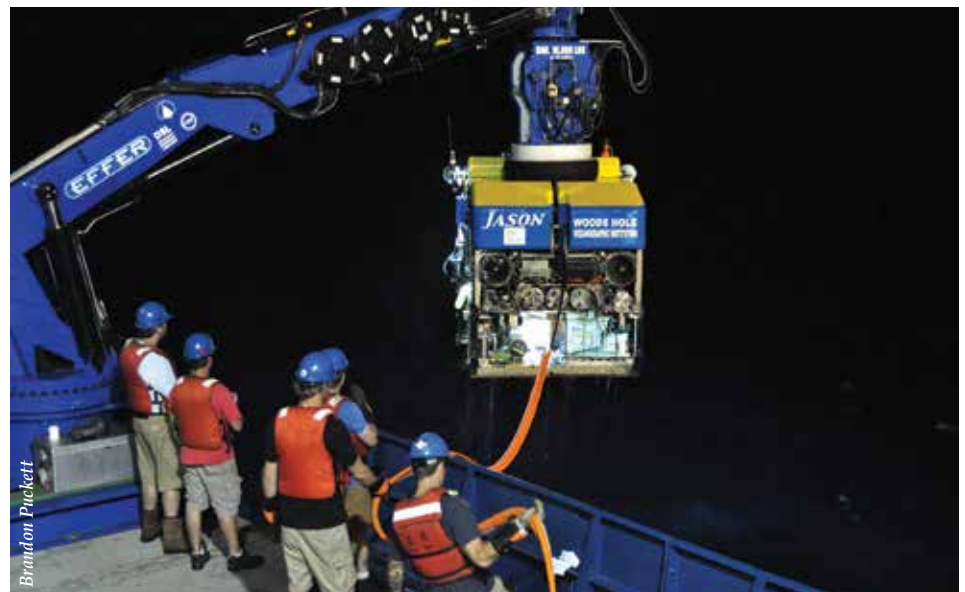
Retrieving the remotely operated vehicle (ROV) "Jason" from a survey of deep-sea hydrocarbon seep communities off Barbados.
